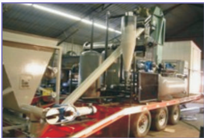
A portable biorefinery for pyrolysis oil production.
