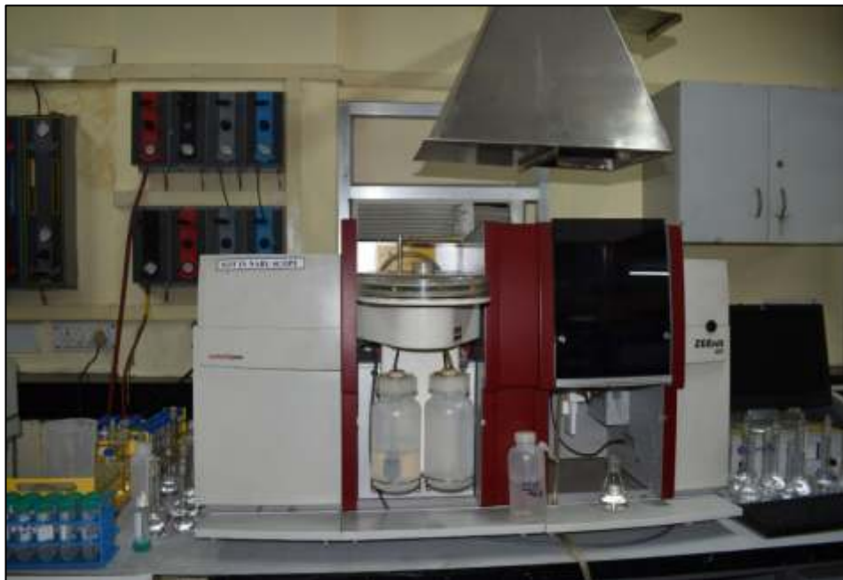
Atomic Absorption Spectroscopy (AAS), modern instrument for heavy metal analysis
