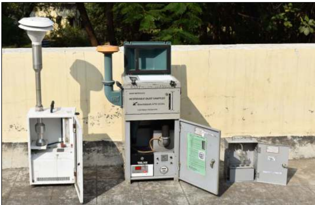
Internal components of fine particulate sampler, respirable dust sampler and impinger box for PM 2.5 , PM 10 , SO 2 and NO x sampling
